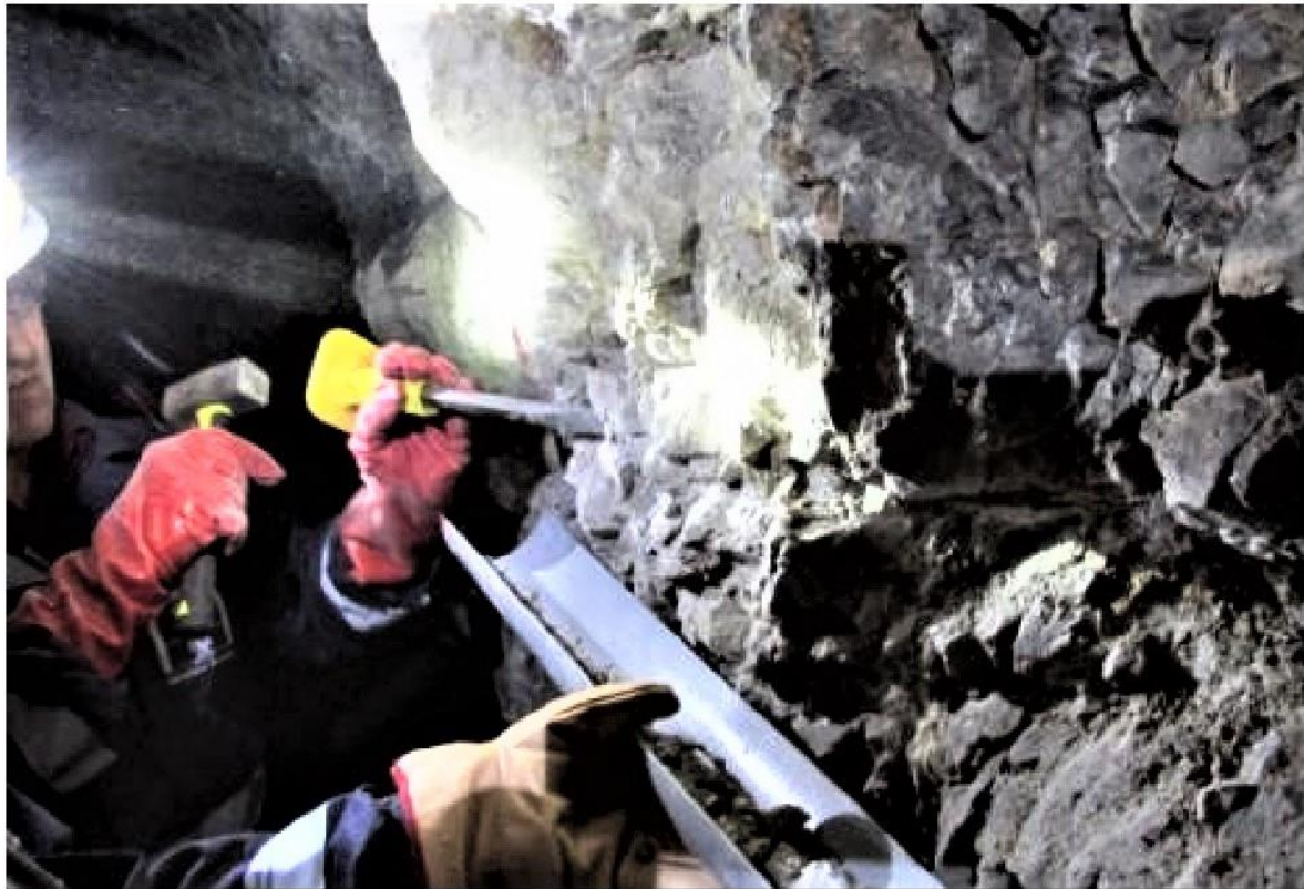
Picture showing collection of a channel sample from the walls of a trench using a metallic slauce as collector.
